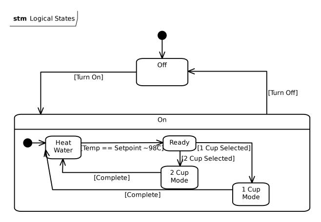
Open the Logical States diagram and use the Toolbox to add the additional substates and transition. Guards for the transitions, shown surrounded by brackets, are added by selecting the transition and adding the guard in the Property Editor.
