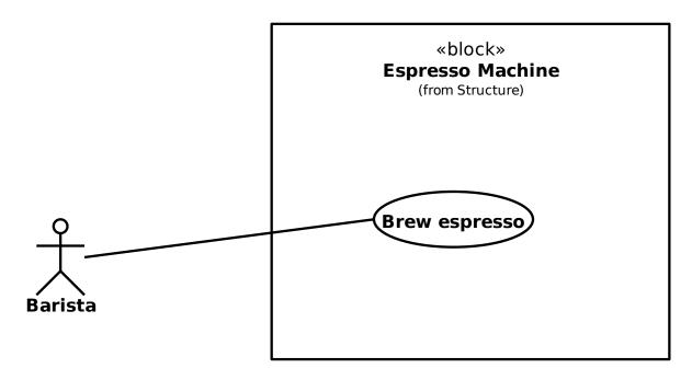
The use case Brew espresso represents a specific functionality or action that the system (the Espresso Machine block) can perform. It describes the steps or interactions necessary to complete the task of brewing espresso, such as selecting the appropriate settings, starting the brewing process, and stopping the process once it's complete.
