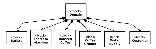
The Barista block is responsible for preparing and serving the coffee to the customers. The Roasted Coffee block contains the types of coffee available for the barista to use. The Coffee Grinder block grinds the roasted coffee beans to the desired consistency before brewing. The Water Supply block contains the water source for the coffee machine, and finally the Customer block represents the person who orders and receives the coffee.
