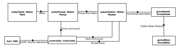
The interactions between the part properties inside the espresso machine are shown as ItemFlows on the Connectors.
