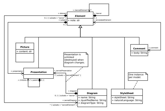
The *Element* base class provides event notification and integrates with the model repository (internally known as *ElementFactory*). Bi-directional relationships are also possible, as well as derived relations.
